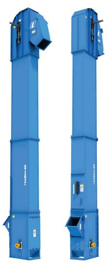
Constructed with the take-up system in the head casing rather than the boot. This design allows for a curved bottom boot to reduce product build up and offers a better seal for fine and dusty materials.
